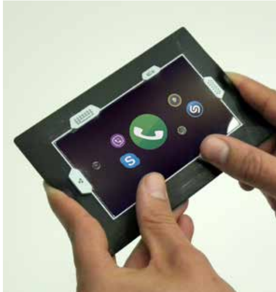
Fig. 3. FLEX with (A) a flexible rim and (B) hardware components around (C) the screen.
